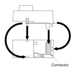
5. Mount the front cover (removed previously) on top of the RS-422/485 Communications Unit, and secure it using the front cover mounting screws. (Do not mount the optional cover.)
