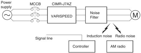
Induction Noise: Electromagnetic induction generates noise on the signal line, causing the controller to malfunction.
