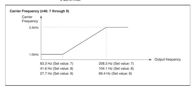
The Inverter cannot maintain rated output current with the carrier frequency set to a value higher than the default one.
