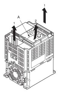
4. Align the Unit with the Inverter's connector, and push the Unit onto the Inverter (so that the 3 catches enter the corresponding holes) until it is securely mounted.
