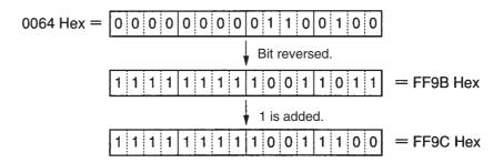
**Note** Whether the data is positive or negative is determined by the parameter set value. The MSB of negative-value data is always set to 1. Data with its MSB set to 1 is not, however, always negative-value data.
