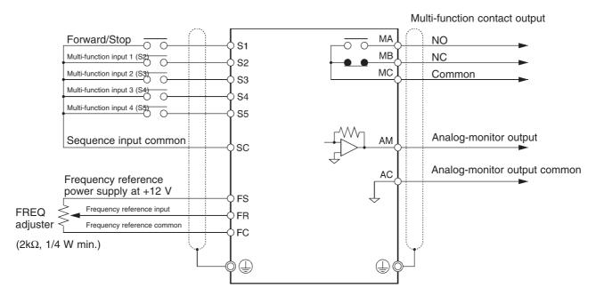
**Note** I/O signals can be connected to a single shielded cable.
