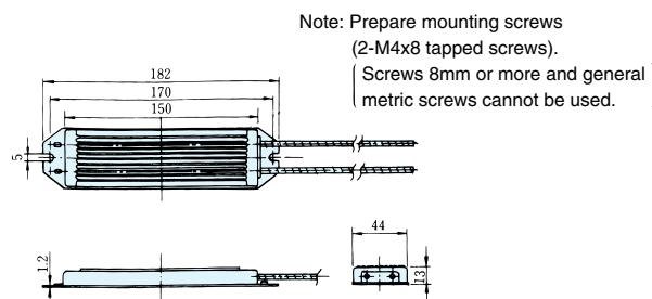
**Braking resistor unit (separately-installed type)**
