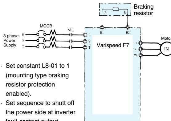
**Connections for braking resistors**
