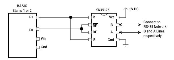
The SN75176 requires 30 mA, therefore we recommend driving only one of these chips from the Stamp's Vdd pin provided no other components require current. Setting RE (Not Receiver Enable) to Low, the R (Receiver) pin is enabled, allowing the Stamp to receive any data coming over the A and B RS485 network lines. Setting DE (Driver Enable) to High allows the Stamp to transmit data over the RS485 network. Vcc and Vdd are electronic terms with the same meaning.
