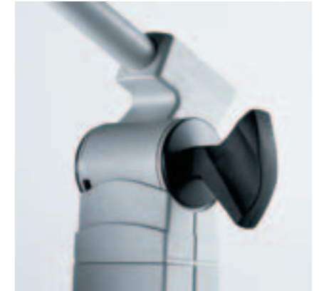
Spring-balanced friction joints with ergonomically designed tommy screws provide for easy adjustment. The luminaire head can be positioned with one hand. When the friction is set correctly, the tommy screws do not require readjusting.
