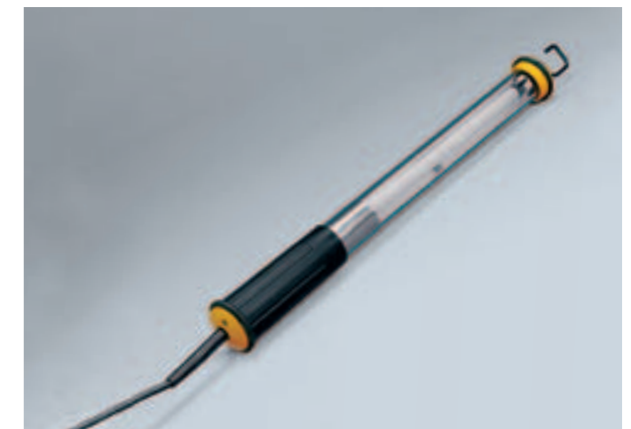
HLE 108 hand luminaire. Jet-proof and dust-proof in accordance with protection system IP 20 or IP 65. Light (under 500 g) and handy. With integrated electronic ballast in the handle.
