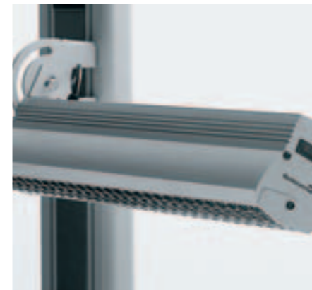
The SAMKC 136 system tasklights are mounted on the vertical side-members of the profile frame. This results in bright, reflection-free illumination with minimal shadow effects. The light emission angles and mounting heights of the luminaires are individually adjustable (mountings not included). Aluminiumised parabolic louvre to eliminate direct glare.
