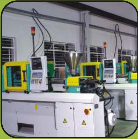
MOULDING MACHINES ARBURG, GERMANY
