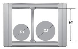
The laying of numerous cables on top of each other or numerous cables or conduits of greatly differing diameters next to each other is only recommended when separators are used.
