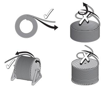
Highly-flexible cables or individual wires with a diameter of up to 6 mm should be combined loose and laid slightly twisted in a cable protection conduit.
