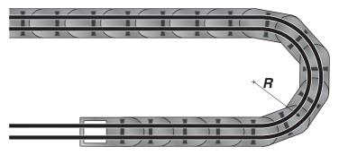
The weight distribution in the chain link should be as symmetrical as possible, i.e. heavy cables/conduits must be laid outwards, with light ones inwards.
