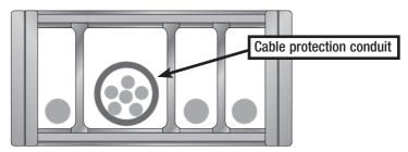
The cable protection conduits must be able to move freely in the frame bridge. A much larger conduit cross section must be selected than the sum of the individual cross sections (max. filling approx. 50 %).
