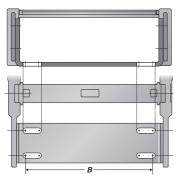
If connection is only possible using mounting brackets (type KA), U-profiles (special articles which are not listed in the catalogue) must be used instead of the standard metal angles in order to ensure stability and permanent absorption of the torques. Please contact us.
