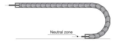
Only with this arrangement is it possible to exclude relative movement between the cables and conduits and the cable drag chain.
