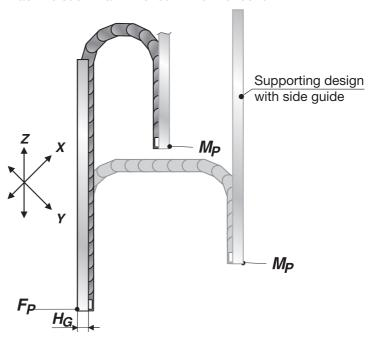
The moving end connection moves in the Y- and Z-directions. The entire system additionally is moved in the X-direction. A lateral guide spanning the entire travel distance is absolutely necessary.
