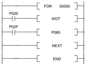
When P020 is on, the current value of WDT is reset and no WDT error occurs. Otherwise, a WDT error occurs and program is stopped.
