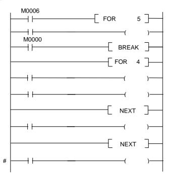
When M000 turns on, exits immediately from FOR  $\sim$  NEXT loop and go to the step #.
