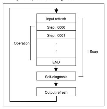
Fig. 2-3 Operation processing of the CPU
